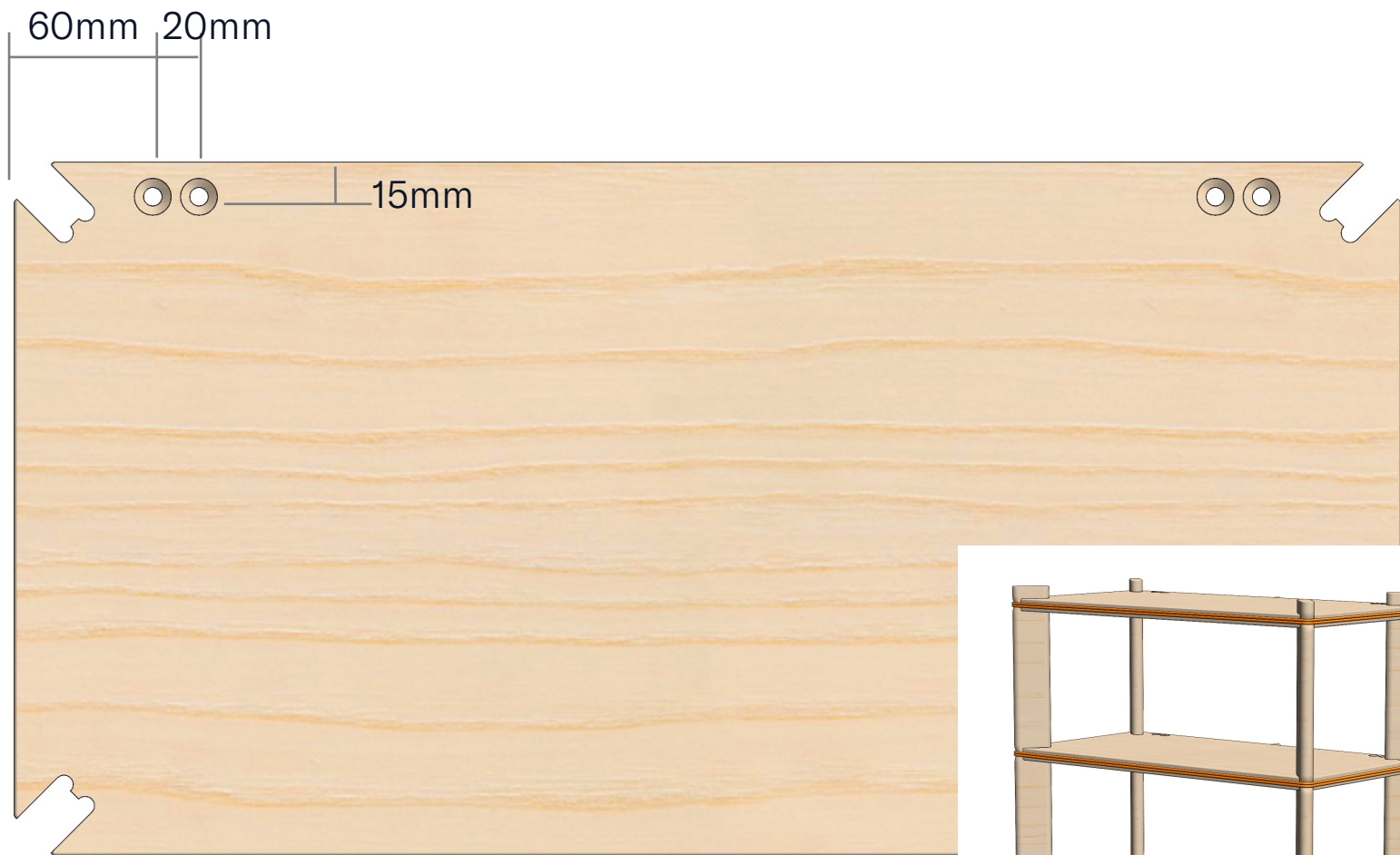
Drilling 4 holes of 6mm diameter like shown in the second lowest board. These are for the diagonal tensioning. Chamfer the edges.
