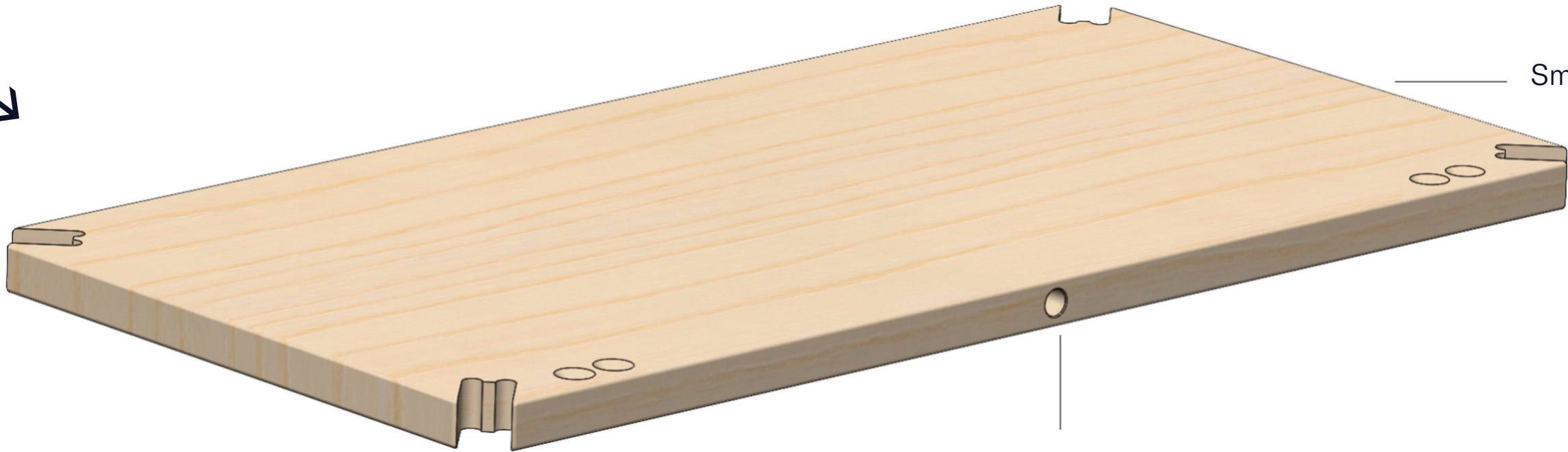
Drilling a hole in the middle of the backside of each board. Diameter: 10mm, 20mm deep.
