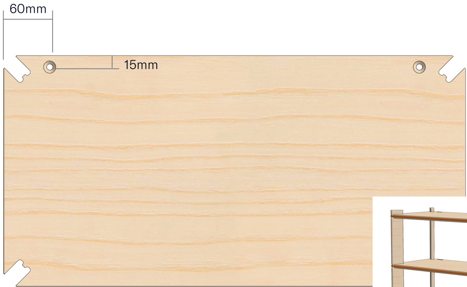
Drilling 2 holes of 8mm diameter like shown in the lowest board. These are for the horizontal tensioning. Chamfer the edges.
