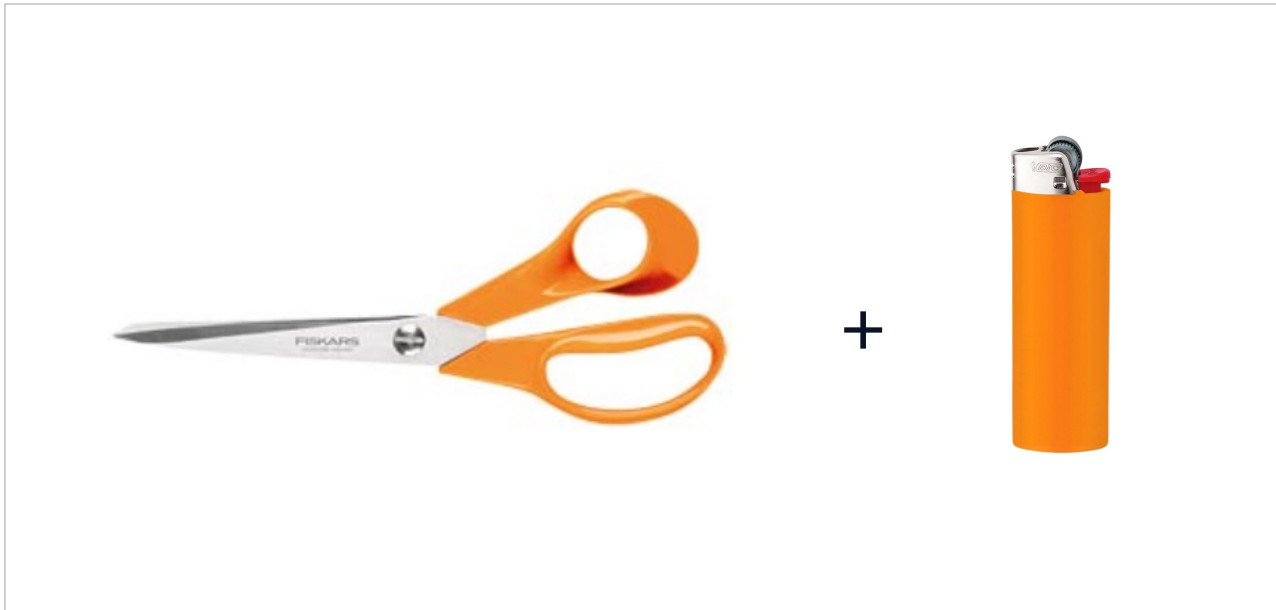
Scissor for cutting the rope and a lighter for melting the ends of the ropes to avoid fraying.
