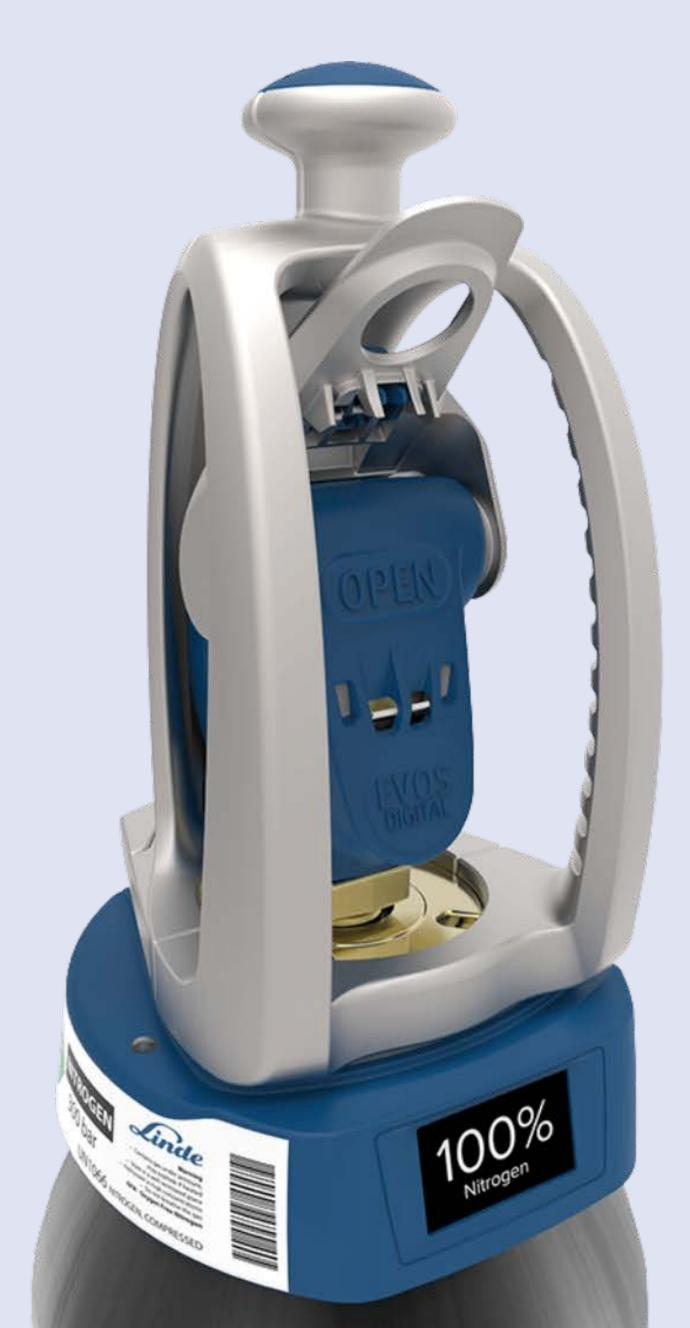
The EVOSTM DCi is an application for all valves across the entire product range which uses sensors to transmit live cylinder position data and gas information including gas type, gas volume, gas flow rate and even cylinder temperature. Using data transmission and storage in the cloud, customers have instant, device-independent access to current and historical gas information.
